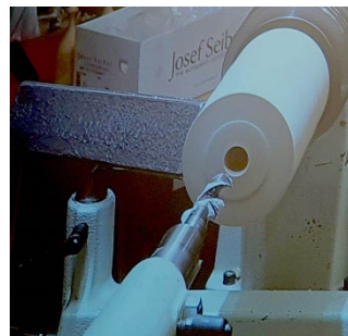
Winding the drill into the blank using the tailstock handwheel
