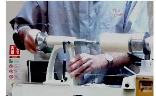
Winding the drill into the blank using the tailstock handwheel
